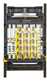
Infinera Line System 2 (ILS2): ILS2 is a 160 wavelength line system to extend the reach between DTNs up to 2500km. ILS2 includes both Raman and EDFA amplification options and provides industry-leading 25GHz channel spacing.
