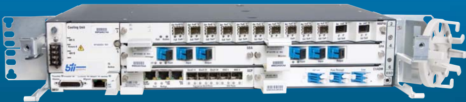
BTI 7060 Dimensions: 2RU | Service Slots: 6 | AC and DC Power Options | Expansion Shelf Architecture Option
